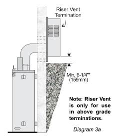
\*Diagrams 3 & 4: As specified in CGA B149 Installation Code. Local codes or regulations may require different clearances.
